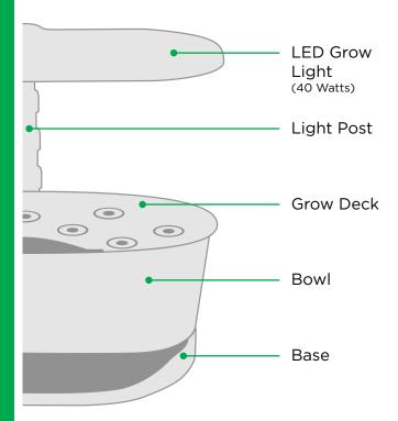
Garden Input: 24Vdc, 2.0A | Adapter Input: 100-240Vac, 50/60Hz Adapter Output: 24Vdc, 2.0A
